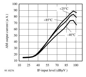
Figure 25. AM-demodulator characteristic vs. temperature
