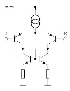
Figure 4. Pin 1 OP<sub>in+</sub>
