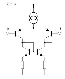
Figure 19. Pin 16 OP<sub>in-</sub>
